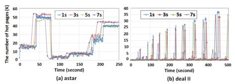
Fig. 10. The number of hot pages under the configuration of different sampling intervals.
