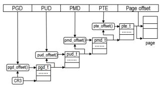
Fig. 1. Four-layer page table under 64-bit operating system.
